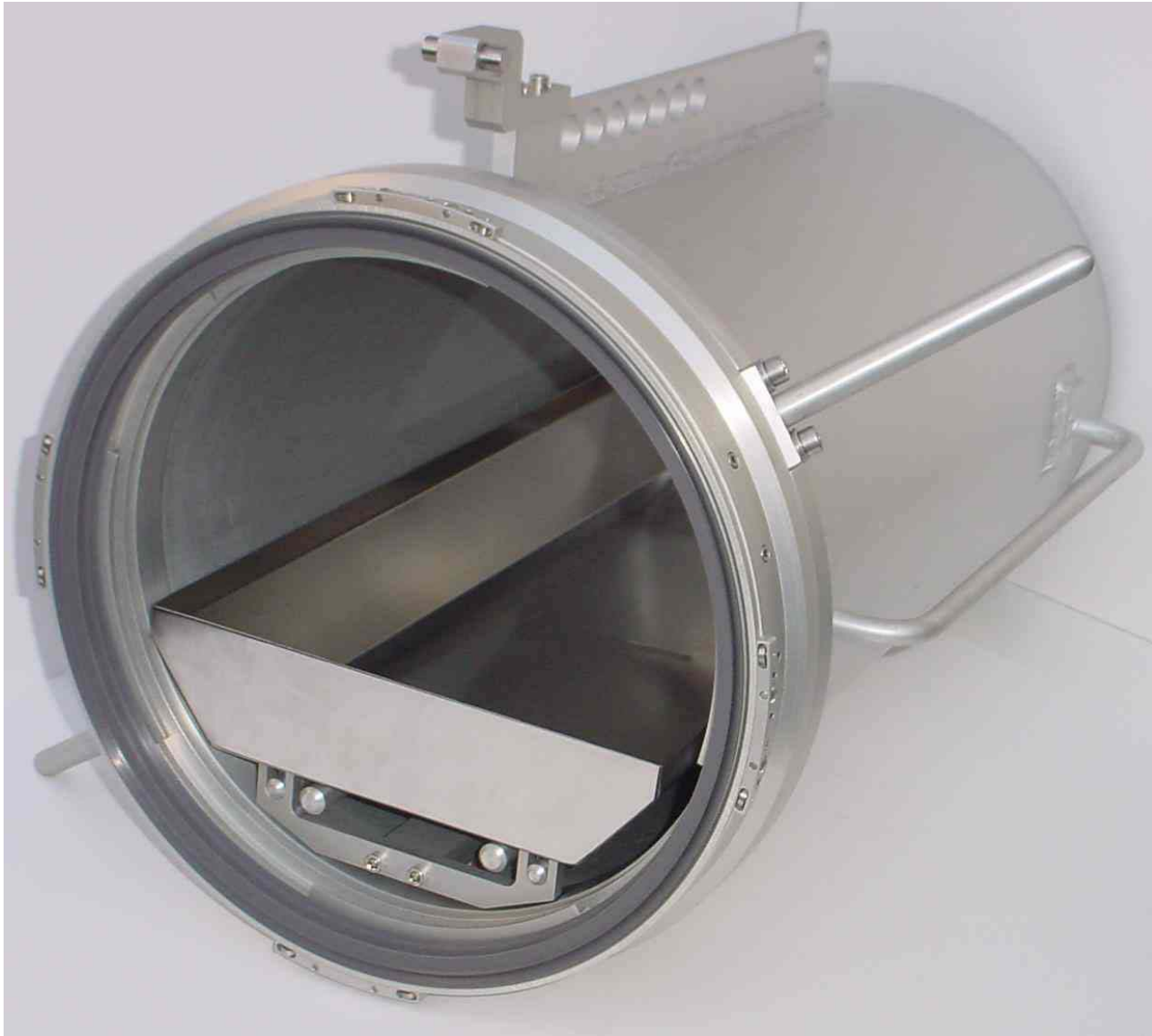
NRC - Tray connected to shuttle shown in retracted position
