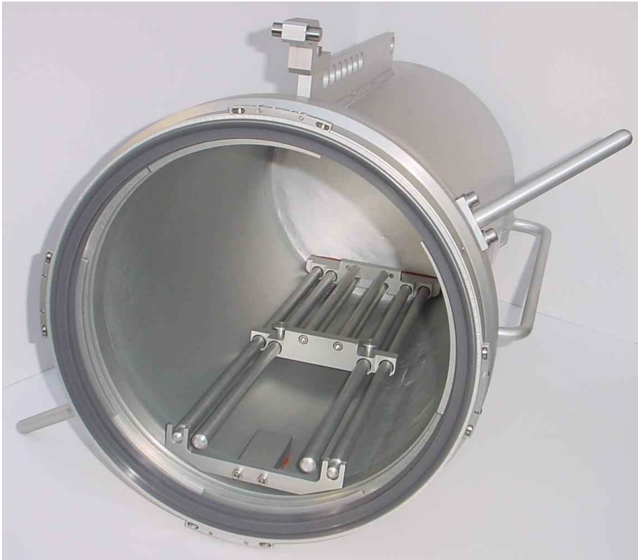
NRC - Beta door removed - Shuttle mechanism retracted
