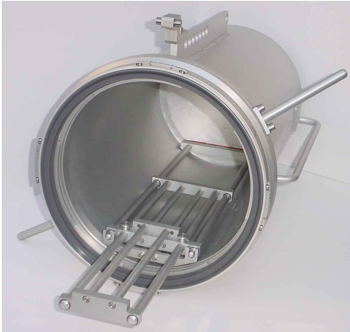
NRC - Beta door removed - Shuttle mechanism extended
